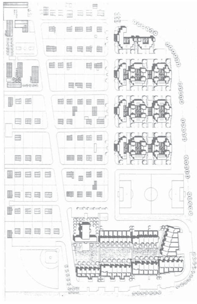
Fig. 29. The site plan for Cabrillo Village illustrates several “democratic spaces.” The grid streets of the old camp and new four-plex units, the common green of the row house development, and the basketball court related to the community building which links all three residential areas.
